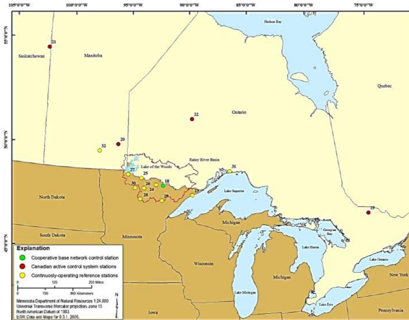
**Figure 3.** Map showing the locations of a National Geodetic Survey cooperative base network control station, four Canadian active control system stations, and ten continuously-operating reference stations that were used to process collected satellite data.
